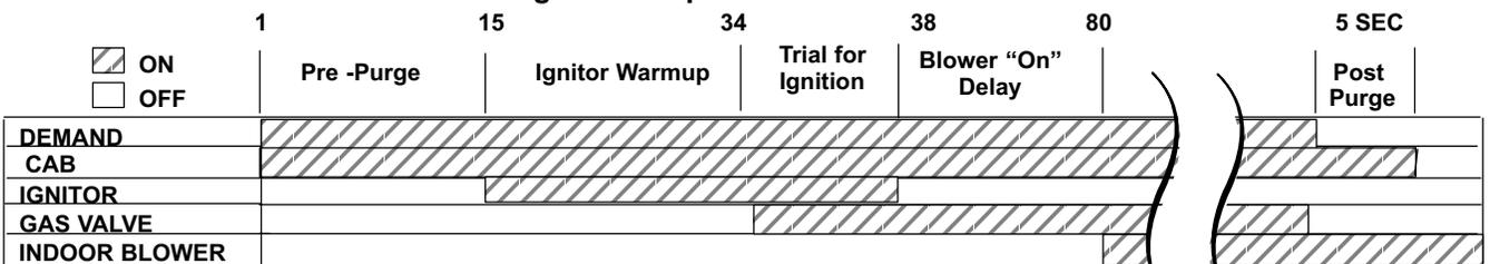
\*Blower on time will be 45 seconds after gas valve is energized. Blower off time will depend on "OFF TIME" Setting.
